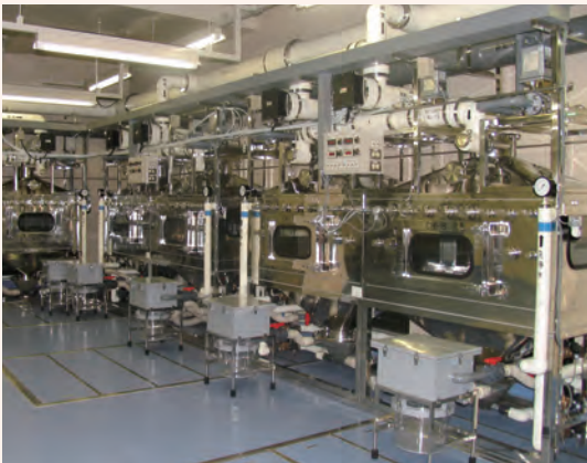
Inhalation Exposure Chamber (Short-term Study)
