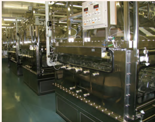
Inhalation Exposure Chamber (Long-term Study)
