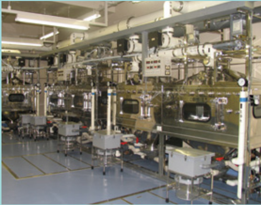
Inhalation Exposure Chamber (Short-term Study)
