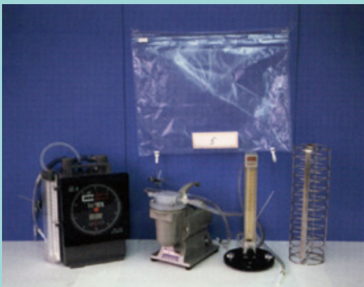
Gas Exposure System (Ames-test) a)
