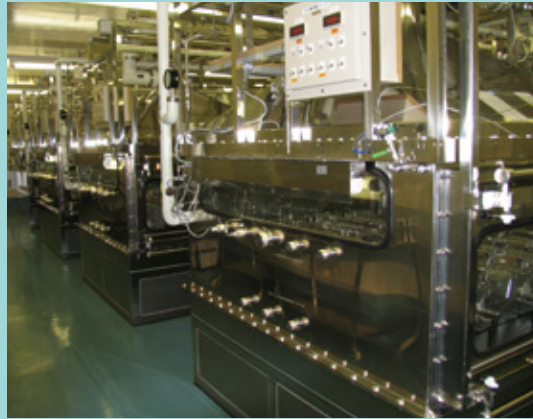
Inhalation Exposure Chamber (Long-term Study)
