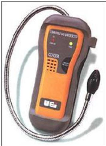
Example of a portable meter that can measure hydrogen sulfide.
