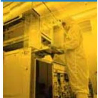
A photomask is aligned and placed on the coated wafer with precision instruments. The wafer and mask are then exposed to ultraviolet (UV) radiation from an intense mercury arc lamp. This causes exposure to the photo resist in places not protected by opaque regions of the mask. With a typical positive photoresist, the areas struck by light undergo a chemical
