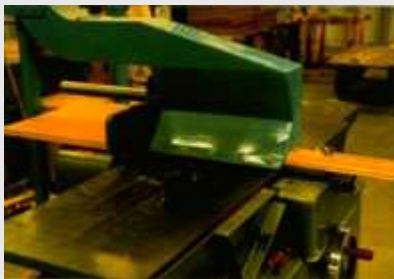
View of timber planer-thicknessing machines after adjustment
