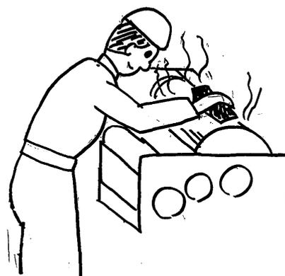
printing devices of the machines at frequent intervals. The cleaner, used until 2006, contained chlorinated hydrocarbons and was highly volatile. It is to be noted that the workers in the plant were engaged longer time in the cleaning process than those in other plants with ordinary printing due to the repetitive cycles.
