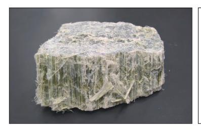
All types of asbestos shown below are totally prohibited in Japan. (Any material containing more than 0.1% asbestos by weight, regardless of type, is illegal.)
